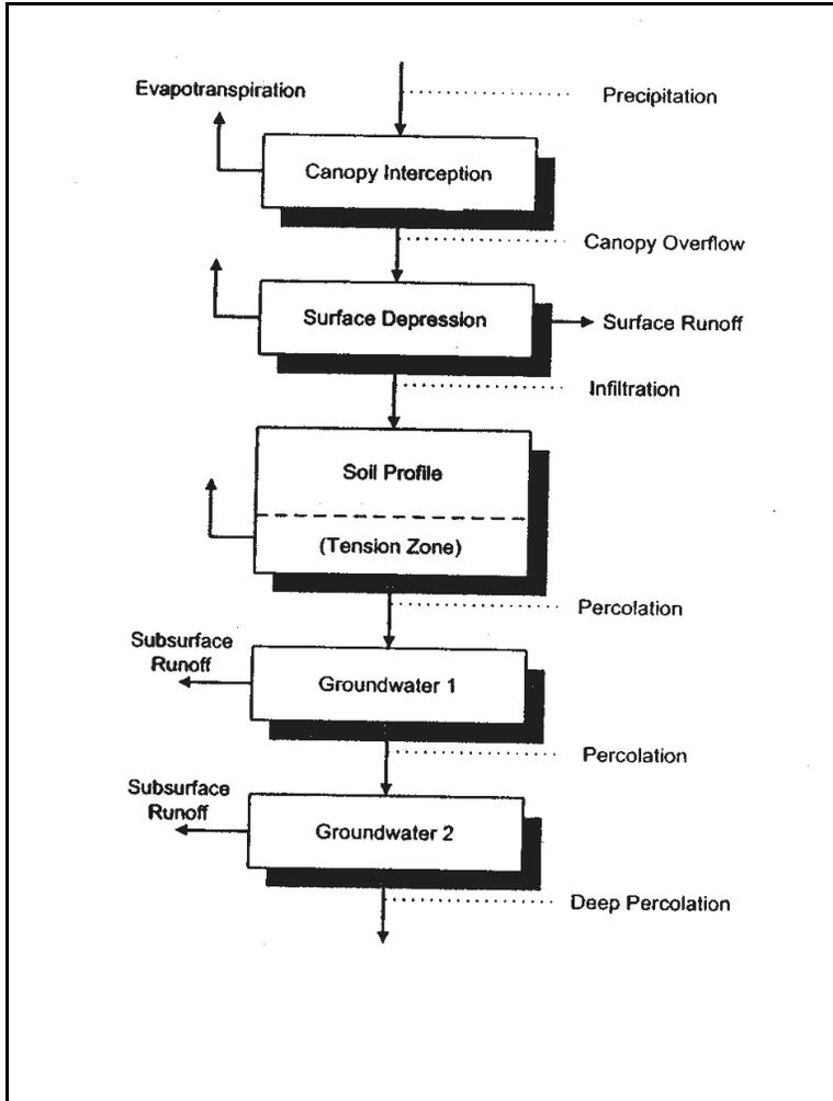
Fig 6 Conceptual View of the Soil Moisture Accounting Method
