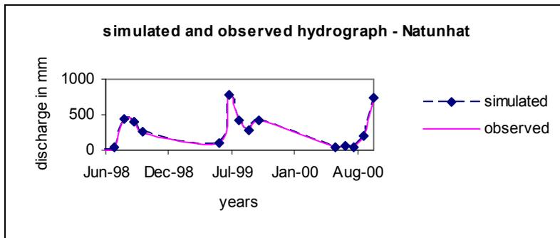
**Fig 3: Simulated and Observed Hydrograph at Natunhat 1998-2000**
